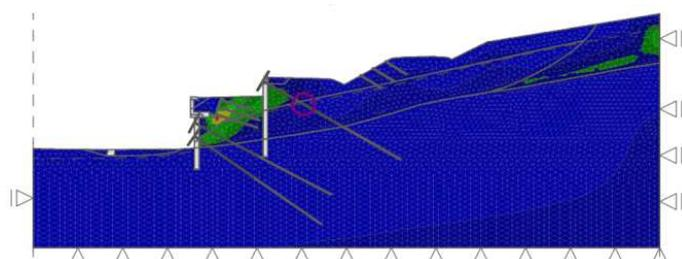
Figure 5. The final stability system of highway
