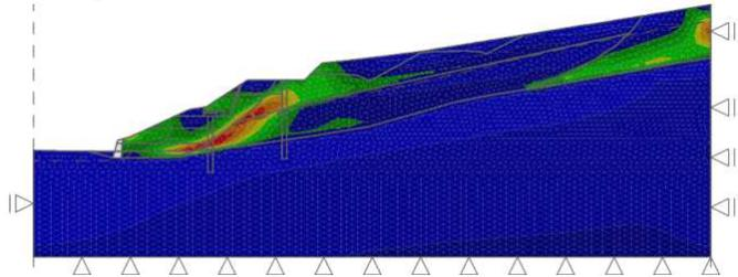
Figure 2. Shape of the shear surfaces for the first construction step (Phase 0 represents the initial stress state)
