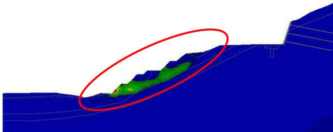
Figure 9. Primary stress state with identified landslide
